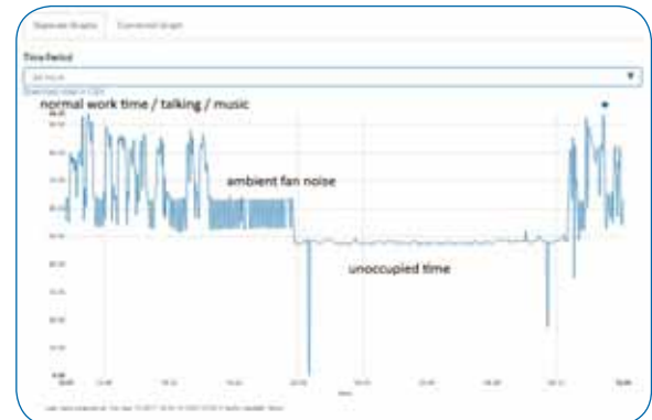
The graph shows a 24 hour sample of noise in an office environment.
